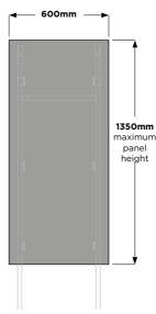
IgPS frames with pre-fitted universal fixing clips are based on these standard panel divisions, however clips can be relocated to suit alternative dimensions. Alternatively IgPS Core Range Units can be purchased without pre-fitted universal fixing panel clips if required.
